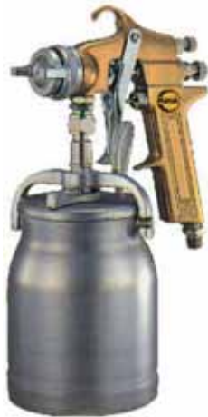
AS-1040-2,0 verfpistool 1,8-1,6mm 1000ml 280L/min, 3,5-5bar
